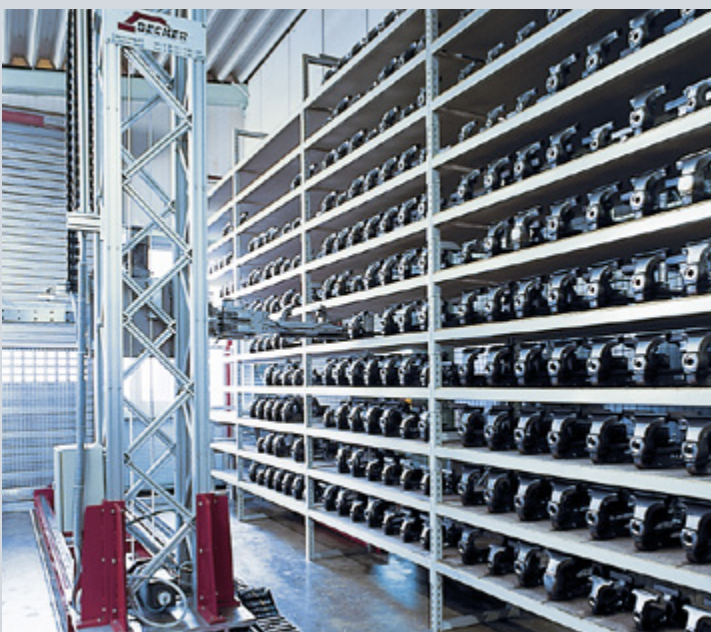
Fully automatic depot and distribution centre
